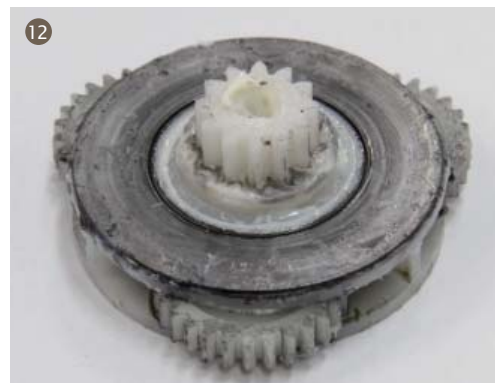
12. Take out filler piece and the epicyclic gear group A
