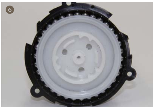
6. Put the steel ball support and 34 roll steel ball into gearbox.
