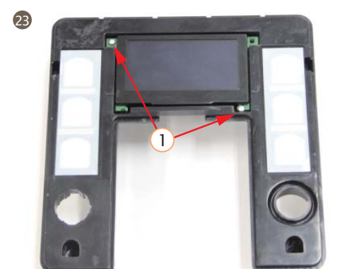
23. Disassemble 2 screws from display screen, and take out the OLED screen
