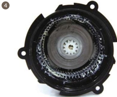
4. Put the already installed epicyclic gear frame A into the gearbox, put 1 filler piece onto epicyclic gear frame A.
