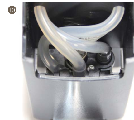
10. Disassemble 1 screw inside the coffee export base, and take out the coffee export group
