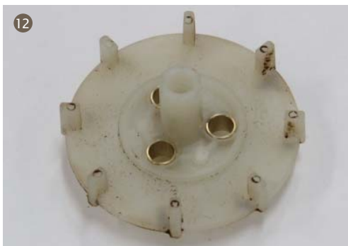
12. Install 3 spring sleeves into the hole of the support lower grinder.
