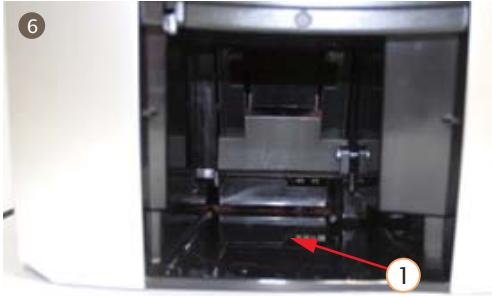
6. Clean the internal machine Clean base
