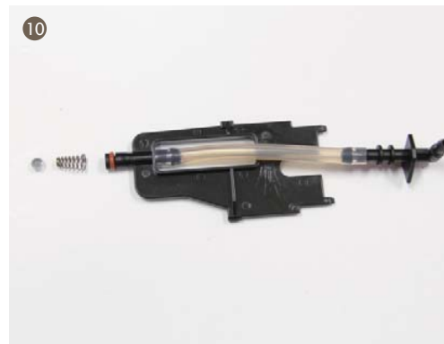
10. Take out the connector, pay attention to the direction of the spring.
