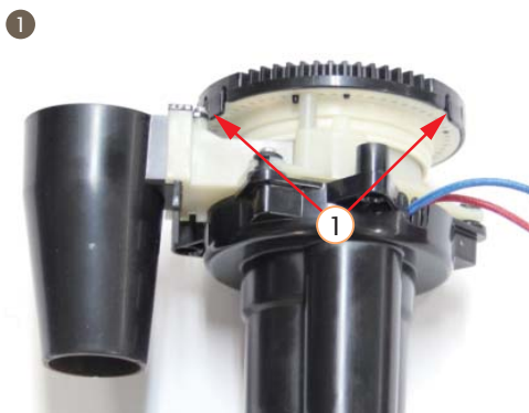
1. Disassemble the 3 hooks from the grinder adjustment sector and take out the grinder adjustment sector
