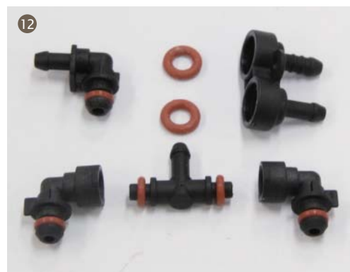
12. Disassemble the connector and seal
