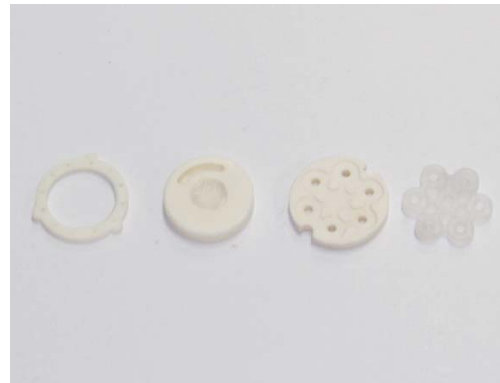
4. Take out water distributor and get out ceramic plate sheet gasket
