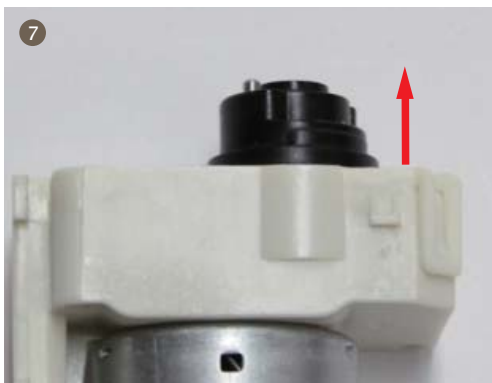
7. Take out the sheave and disassemble the microswitch
