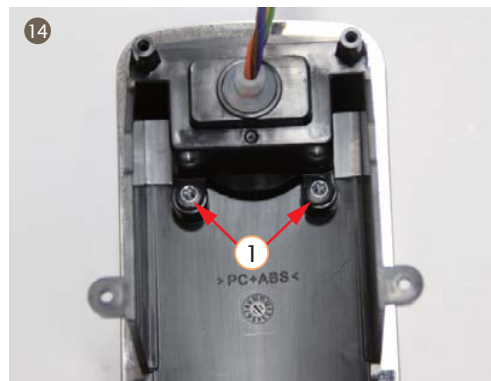
14. Disassemble 2 screws from the backside of the touch screen decorative cover; take out decorative plate and smokebell
