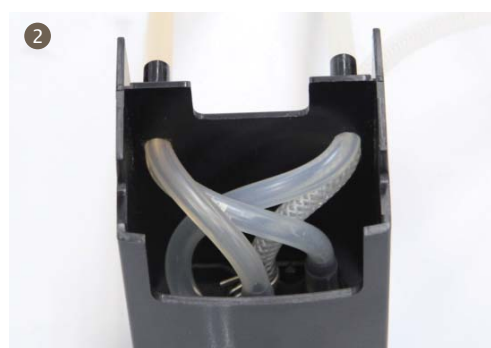
2. When installing silicon pipe, please note the position of every silicon pipe inside the hole of the coffee export.
