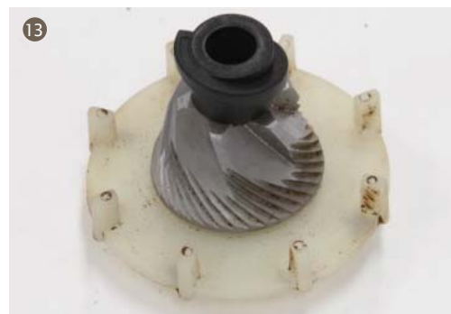
13. Install the screw pin worm drive and conical burr to support lower grinder.
