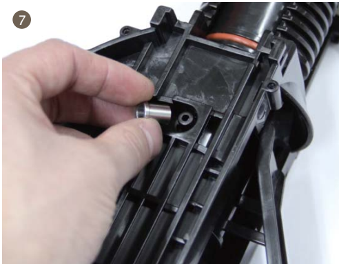
7. Take out left and right pull plate and pull plate sleeve
