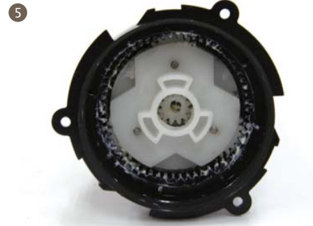
5. Put the already installed epicyclic gear frame B into gearbox.
