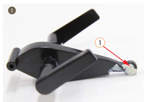
1. Install the piston and release link into the coffee brewing unit, oil(MI-setral-61B) coating position should be as the picture shows.
