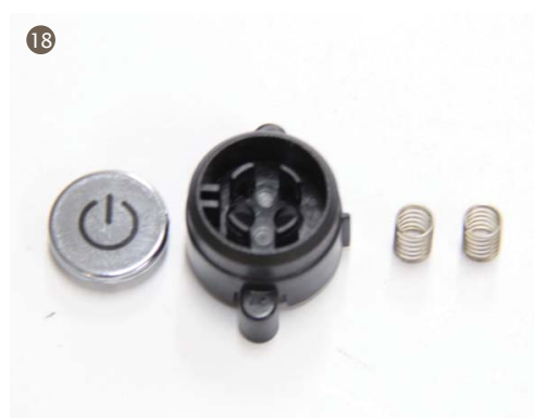
18. Take out the spring and the power button, and disassemble power button decorative cover
