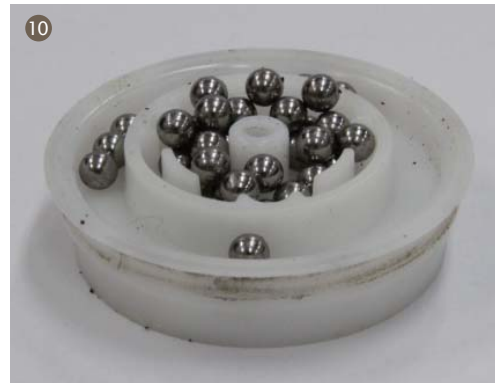
10. Disassemble steel ball support and 34 pcs steel ball
