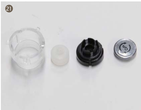
21. Take out silica gel, clean buttons and smokebell, and clean the power button decorative cover
